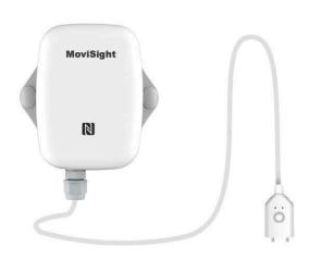
MS700-SLD is a compact spot leakage detection sensor for detecting presence of water (or other liquids) and transmitting alarm using LoRaWAN<sup>®</sup> technology. With this low power consumption technology, MS700-SLD can work up to 5 years with 4000 mAh battery. Combining with MoviSight
