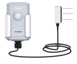
MS800-SMTC is designed for measuring soil moisture, temperature and electrical conductivity in harsh environments and transmitting data using LoRaWAN® technology. With this low power consumption technology, MS800-SMTC can work up to 10 years with 19000 mAh battery. Combining with MoviSight LoRaWAN® gateway and MoviSight IoT Cloud solution, users can manage all sensor data remotely and visually.
